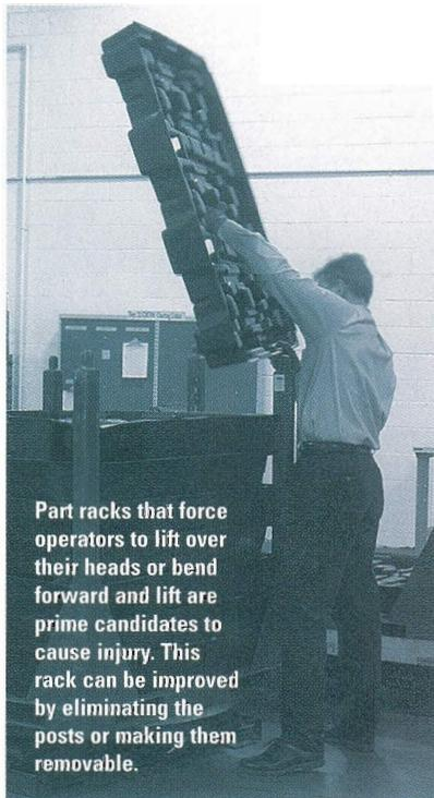
Part racks that force operators to lift over their heads or bend forward and lift are prime candidates to cause injury. This rack can be improved by eliminating the posts or making them removable.
